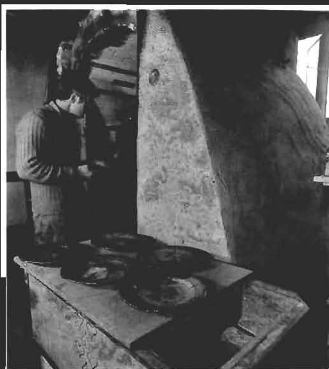
Top Waxed foot rims are dipped into grog prior to stacking; the particles act as ball bearings, easing firing shrinkage.
